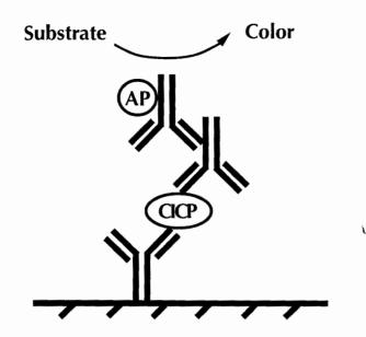
pNPP substrate; absorbance read at 405nm
