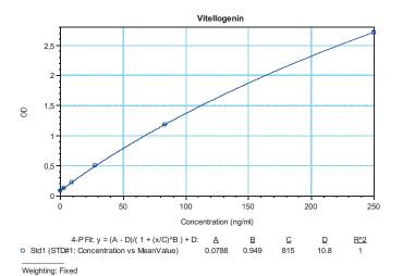
Figure 1 Standard curve by using a 4-parameter curve fit (4-PL).
