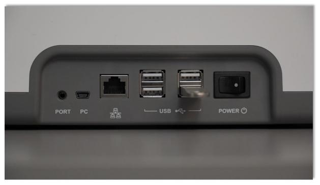
The prepared USB stick is now inserted into one of the four free slots on the F200 and the device is started.
