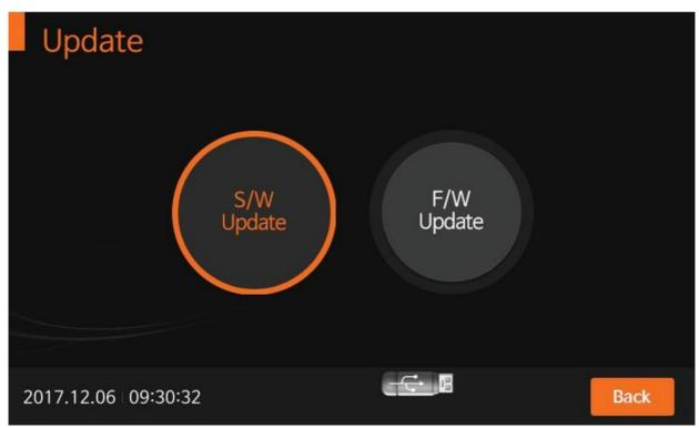
The update is installed after approx. 90 seconds. Please restart the device and remove the USB stick. Your device is now up to date. After the restart, the latest software version is displayed in the bottom right corner of the screen.
